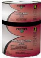
6455/044 Metal Primer is a two component, self-etching wash primer for use only on bare metals including steel, stainless steel, cast iron, copper, bronze, galvanized steel, lead, and aluminum. It forms an excellent adhesive bond to metal hulls, keels, centerboards, and other underwater running gear, and can be used above or below the waterline. Metal Primer can be over coated with epoxy primer, tie-coat primer, topside enamels, or antifouling paint.
